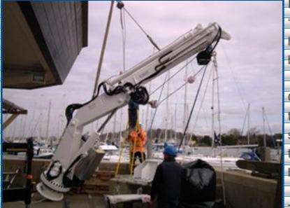
I hope you agree that the resultant pedestal telescopic boom hydraulic winch crane with the splendid marque of 'Iron Fist IFG 26000 ET2' appears imposing and business-like. Built to full marine specifications, Iron Fist cranes have been used for many years in military and fishing vessels and on jetties, so with proper maintenance by our boatmen, we expect it to last us well over 20 years.
