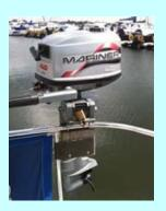
Mariner 4 hp 4 stroke outboard motor.
