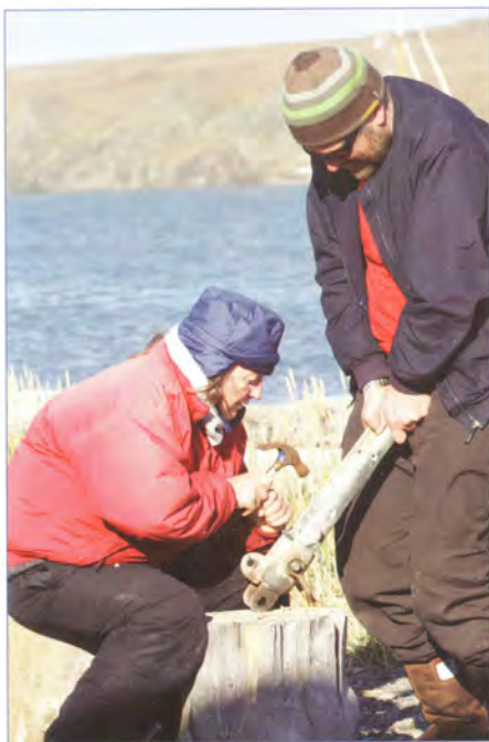
Fabricating a replacement gaff
