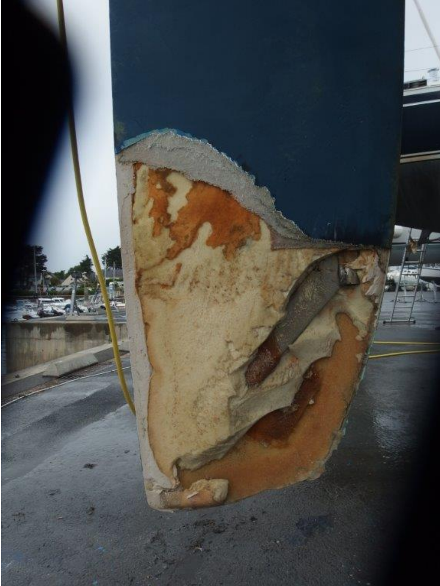
Rudder damage when ANAKAO was lifted out 5 days later at Port Cruesty.
