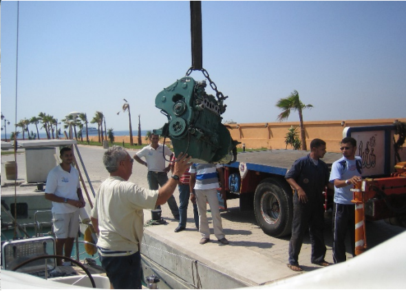
Removing the old engine in Hurghada, Egypt
